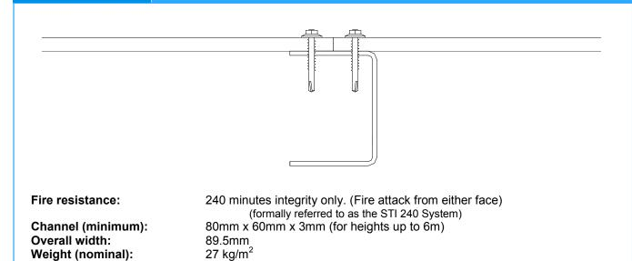
Perimeter channels fastened to surrounding construction with M10 or M12 all-steel expanding anchors (or equivalent for alternative types of supporting construction) at 500mm maximum centres.
