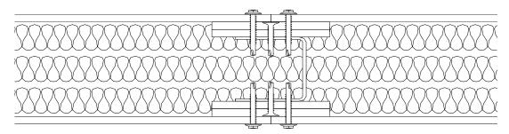
240 minutes integrity - 240 minutes insulation. (Fire attack from either face) Fire resistance:
