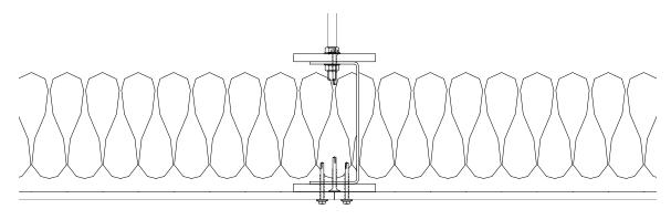
Fire resistance: 240 minutes integrity & insulation. (Fire attack from below)
