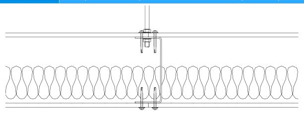
Fire resistance: 240 minutes integrity – 120 minutes insulation (Fire from above or below)
