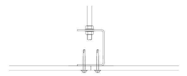
Fire resistance: 240 minutes integrity only. (Fire attack from above or below)
